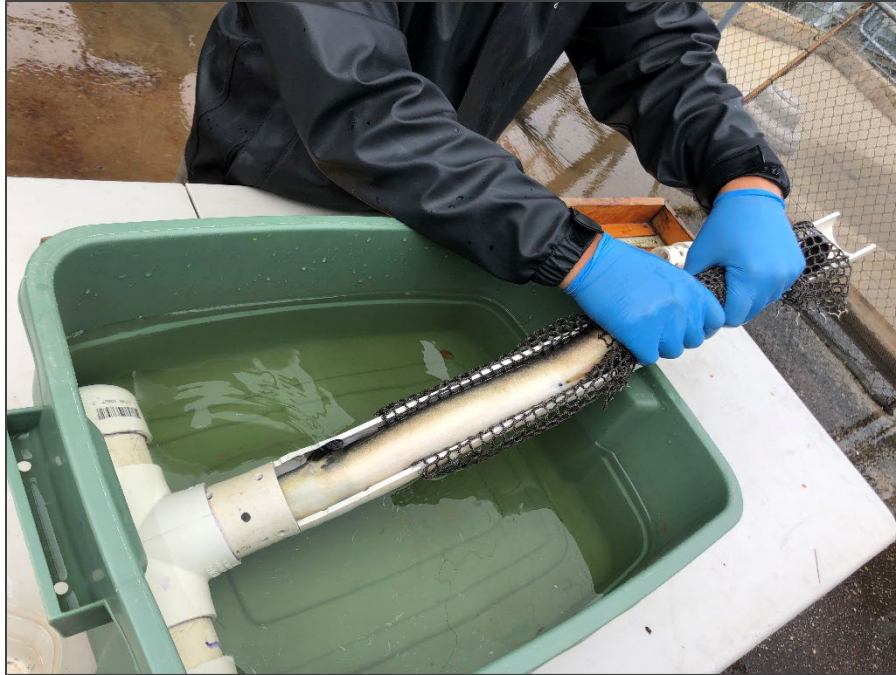
Figure 2-6 Restraint Device for Holding and Positioning Adult Silver Eels during Radio-Tagging*
